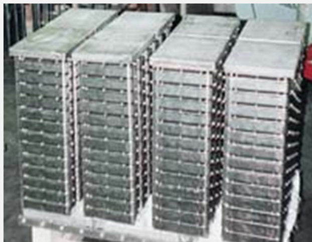
Fig. 6: Prepared plate heat exchanger load
